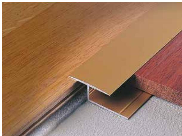
WOODTEC LG profiles are specifically designed to join two adjoining floating wood floors. The size and shape of the profile section allows for differential movement typical of wood flooring. Its smooth top surface fits under doorways making it perfectly suitable for thresholds.
